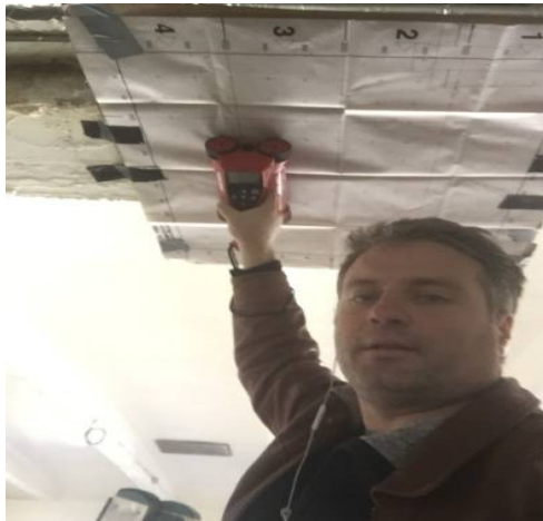
FIG.1 2 SCANNING ELECTROMAGNETIC METOD --- STEEL : 4 BARS 16-18MM + ETR.8MM / 15 CM
