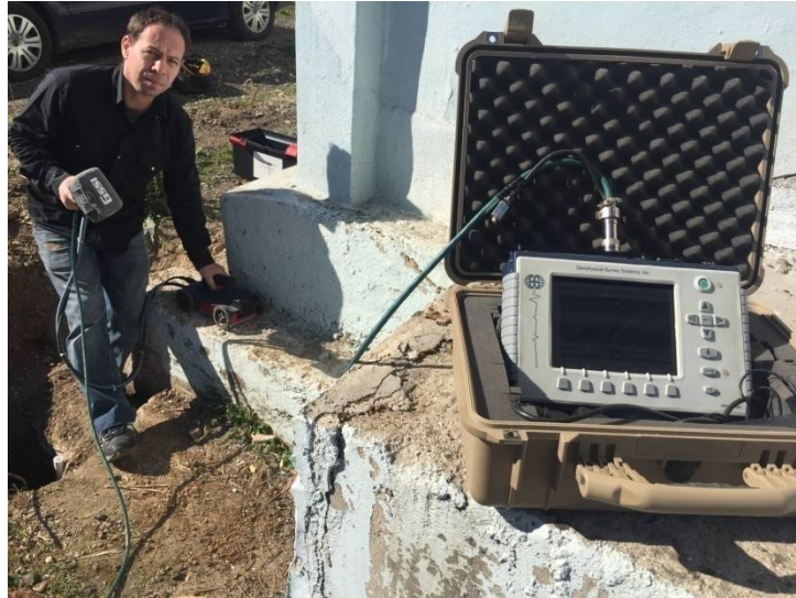
FIG 5 .GPR TESTING WITH 2600 MHZ ANTENNA -FOUNDATION REINFORCEMENT STUDT
