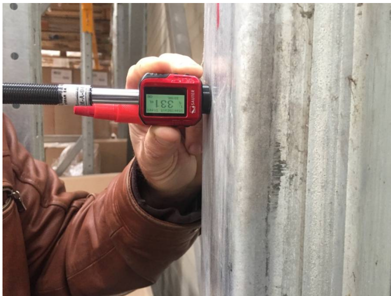
FIG 8.STEEL TESTING WITH DUROMETER-LEEB TIPE TEST
