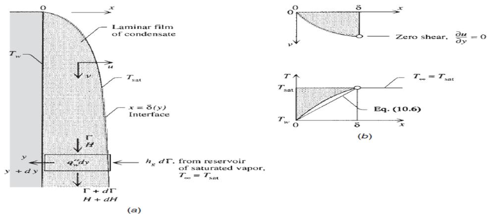
**Figure 2.2. Laminar condensation film from a saturated vapor tank [Bej.2013]**
