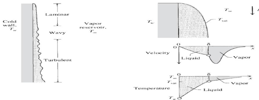
**Figure 2.1. Flow patterns of a condensation film on a vertical surface (Bej.2013)**
